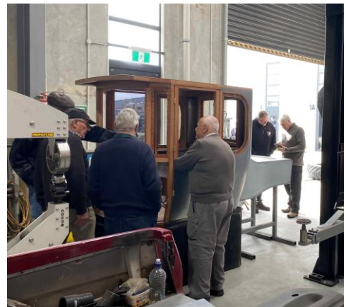
Veteran Panhard body being constructed
