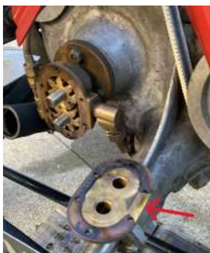
Oil pump gasket failure on the 1909 Wolseley Siddeley
