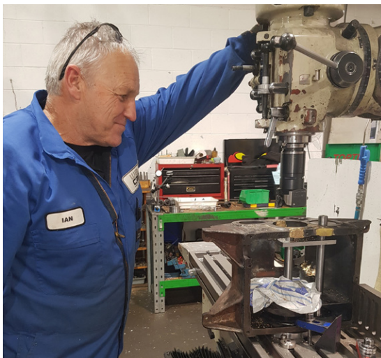
Ian at Wecan Engineering boring the gearbox rear bearing holder
