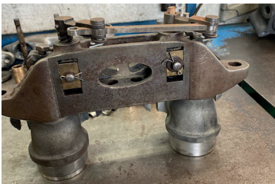
Overhead inlet variable controlled valve block, one of 2.
