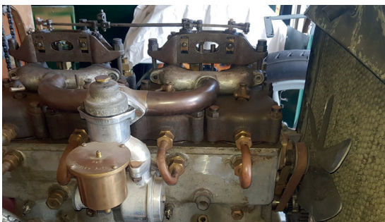
Note the exposed valve gear on the top LHS of motor.
