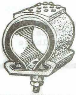
Left. early tyre tread showing old type "Clincher" rim.
