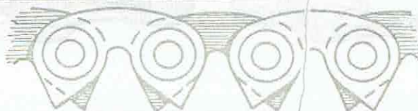
Early transmission chain : Reynolds silent chain.
