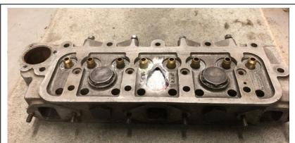
Unsuccessful attempt at repairing the Derrington head. The top section was cut open, but this still didn't allow enough room to gain access the full length of the crack.
