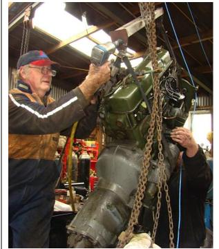
Out it comes – photo shows Ivan's device for tilting the engine as it comes out.
