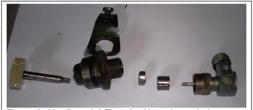
The speedo drive dismantled. The seal and its retainer are in the centre.
