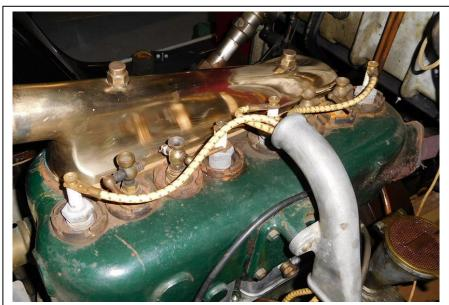
The water manifold on top of the Veteran block. The water staining can just be seen around the valve plug second from rear.
