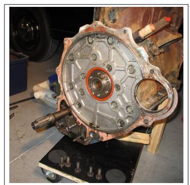
18/85 power unit with the clutch and flywheel removed. The damaged shaft is the one on the left.
