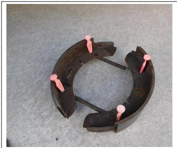
Return springs held in place with pegs for reassembly
