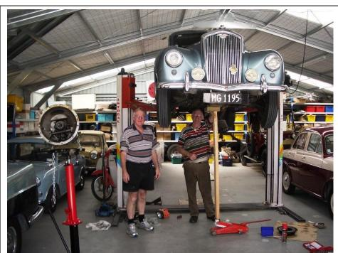
Tony (left) and Graham mid-way through a clutch replacement on Tony's 6/80. The gearbox is on the transmission jack (left)
